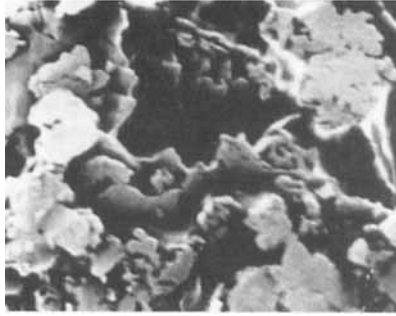
FIGURE 5 SEM photograph of toluene extracted sample of 50:50 AU:CSM blend, prepared by masterbatch technique ( \times 800 ).
